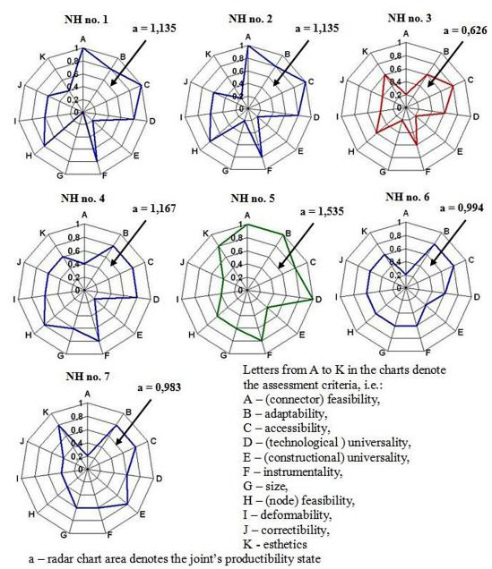
Fig. 2. A set of radar charts for the hybrid nodes assessed [5]
